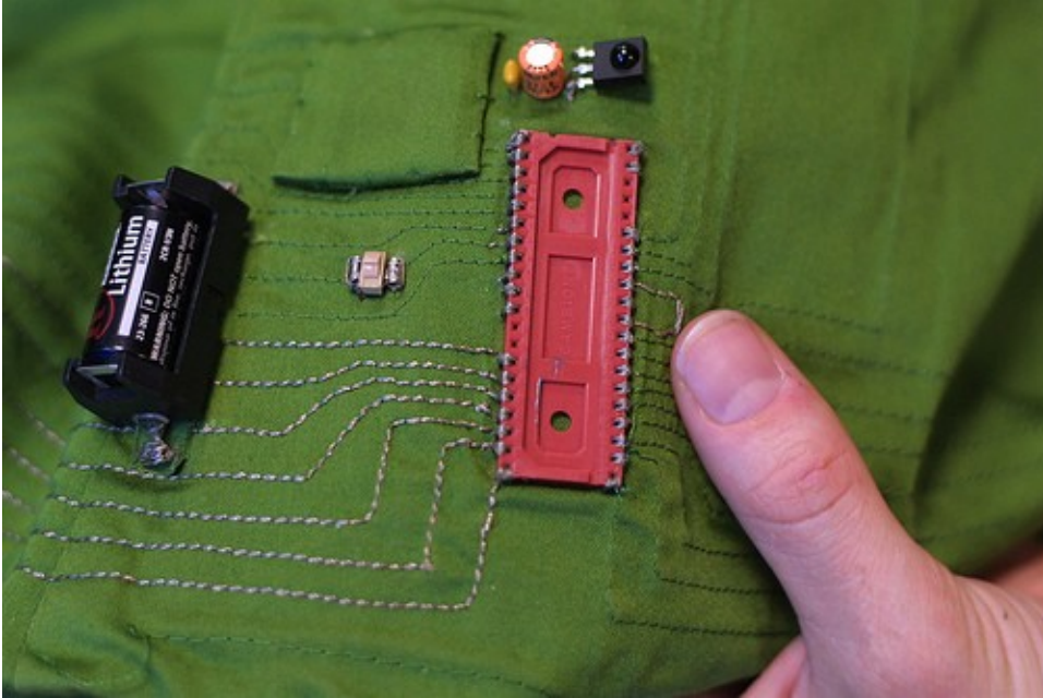
9 Leah Buechley, a soft circuit sans chip previous to the Arduino LilyPad (Photograph provided by Jean-Baptiste Labrune)
