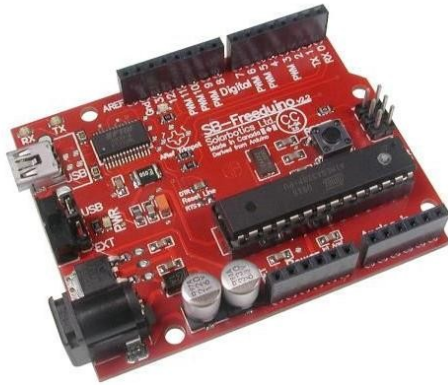
4 The Freeduino , 2.7 in. x 2.1 in. (Photograph provided by solarbotics.com)
