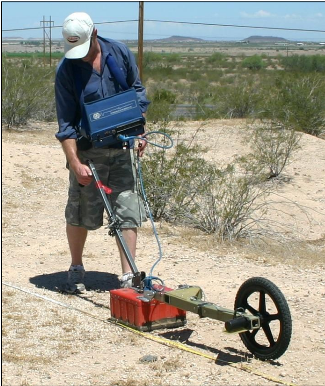
Figure 1. A GSSI Inc. SIR-3000 system with an attached survey wheel for distance measurement. The 400 MHz antennas are positioned in the fiberglass box. Antennas that transmit radar waves into the ground are connected by a cable to the control box for immediate viewing and digital recording to disk.
