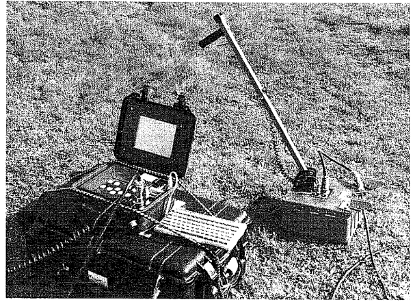
Figure 7.1. The Geophysical Survey Systems Subsurface Interface Radar (SIR) system, Model 2000. The radar control box contains a computer for data collection, processing, and data storage and a computer screen. The radar signal is transmitted to and from the computer by cables, which are attached to the 400-MHz antennas in this photo. Reflection data are visible on the computer monitor during collection and processing.
