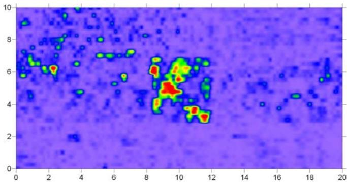
Figure 4: Amplitude maps of the Illinois house floors using the 400 MHz antenna when the ground was extremely wet.
