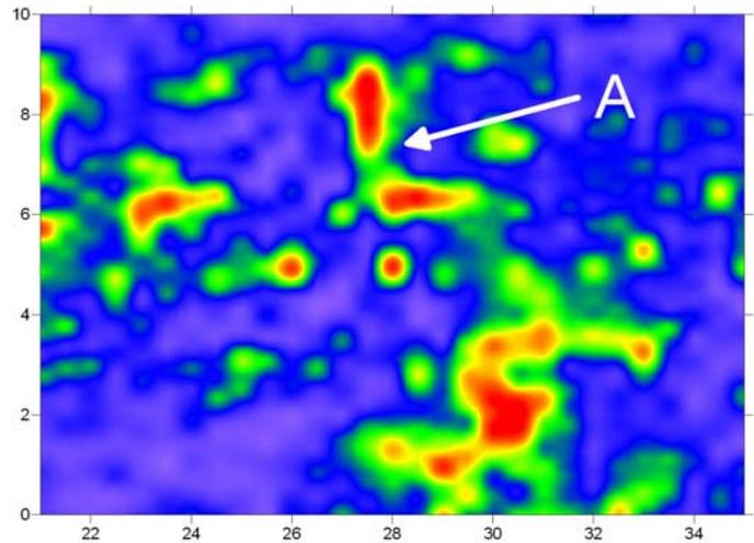
Figure 9: Amplitude map from 1.5 meters depth collected with ground was wet. The wooden beams at (A) are now visible.
