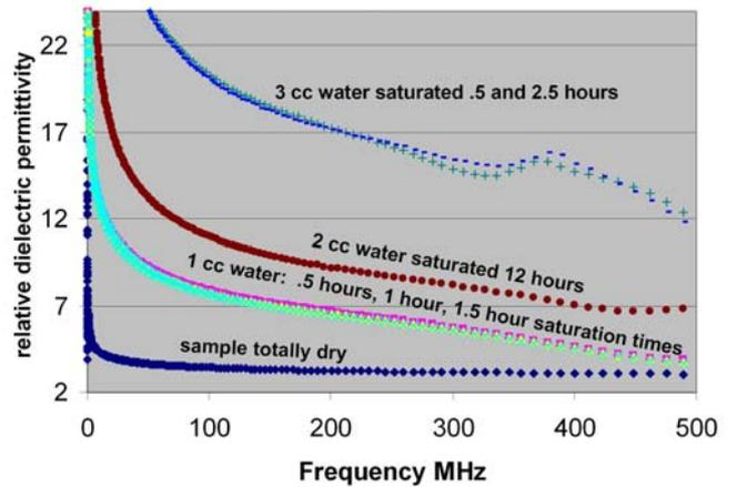
Figure 5: As small amounts of distilled water are added to a 13 cc silty clay sample from the Illinois site, and allowed to sit for varying amounts of time, the RDP increased dramatically.
