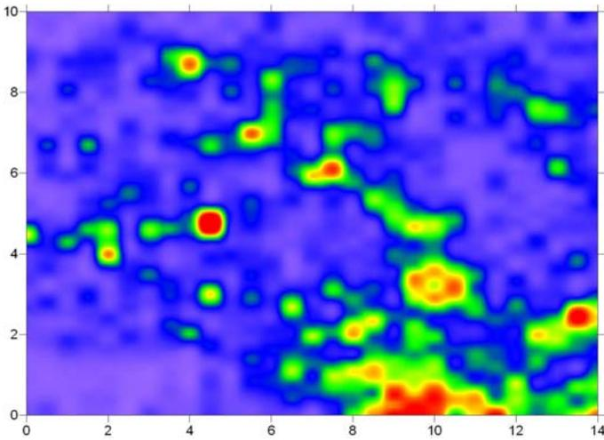
Figure 7: Amplitude map at the Washington test site from 1.5 meters depth. Data were collected when the ground was dry.
