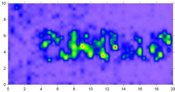
Figure 3: Amplitude map of the 400 MHz frequency reflection data over the house floors shown in Figure 1 when the ground was dry.
