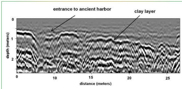
Figure 2. Reflection profile across an ancient harbor in Israel. Homogeneous near-shore sand overlying the clay produces very few reflections. A gravel layer below the clay layer produces many hyperbolic reflections, generated from each large gravel clast. In this profile the entrance to an ancient harbor, dredged through the clay and gravel, can be seen as a deep incision through those layers.
