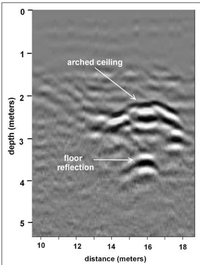
Figure 5. 270 MHz reflection profile across an underground church in Tunisia, which shows much the same reflection features as modeled in advance (Figure 4).
