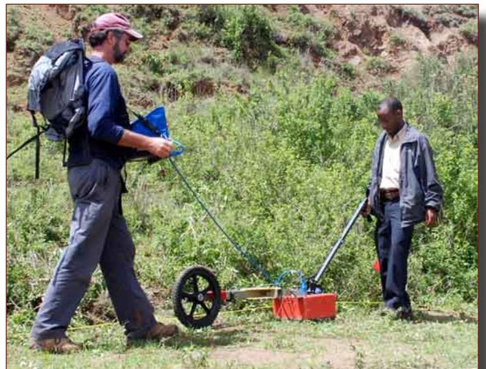
Figure 1. Collecting GPR data using a GSSI SIR-3000 system and 400 MHz antennas attached to a survey wheel.
