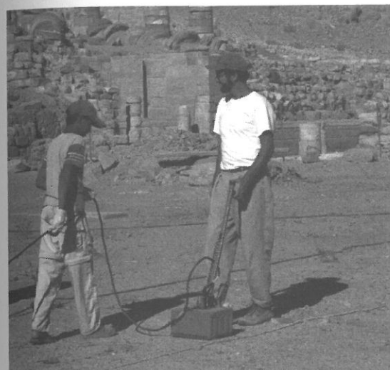
2. A 400 MHz GPR antenna was used to collect reflection data at the Lower Market Site in Petra, Jordan (L. Conyers).
