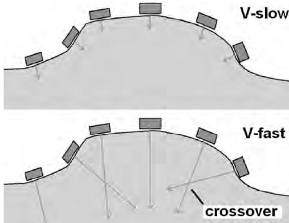
Figure 1. Geometry of vertically transmitted radar waves from a tilted antenna illustrating why topographic and tilt corrections are necessary. Higher velocities can also create conditions where reflection trace 'crossover' occurs.
