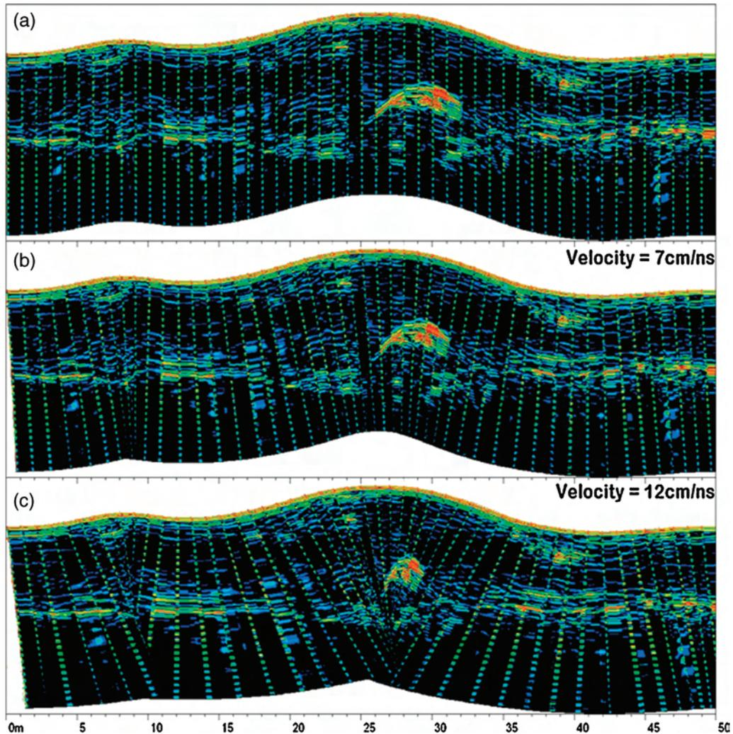
Figure 2. An example of topography and tilt corrections applied to the same reflection profile. The upper figure (a) has no correction for tilt but the lower two are corrected using velocities of  $7 \text{ cm ns}^{-1}$  (b) and  $12 \text{ cm ns}^{-1}$  (c).
