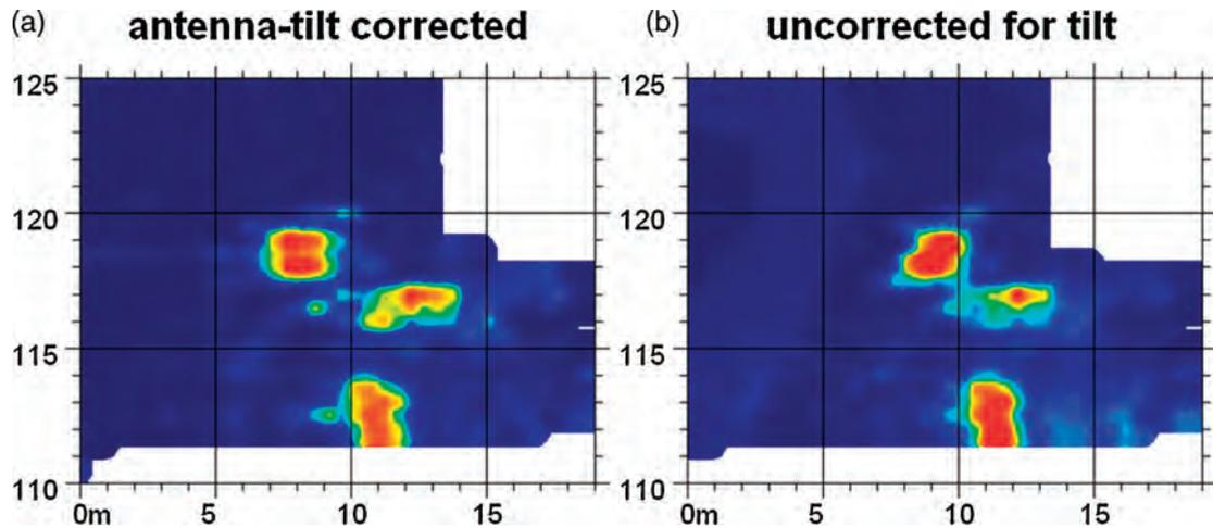
Figure 4. A comparison of amplitude time slices made from topography and tilt corrected reflection profiles (a), with those that were made from uncorrected profiles (b). These amplitude time slices illustrate reflections from the chamber ceiling from 3.5–4 m below the ground surface of Ikime Burial Mound number 7, Miyazaki City, Japan.
