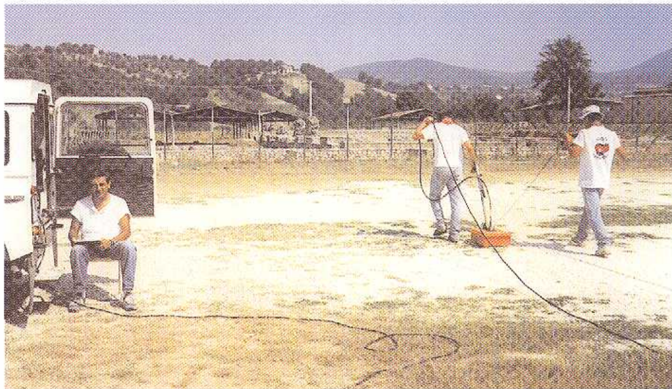
Collecting GPR data at the Forum Novum, Italy. The antenna is dragged across the field. Note that there are no surface indications of the archaeological features that are preserved below.
