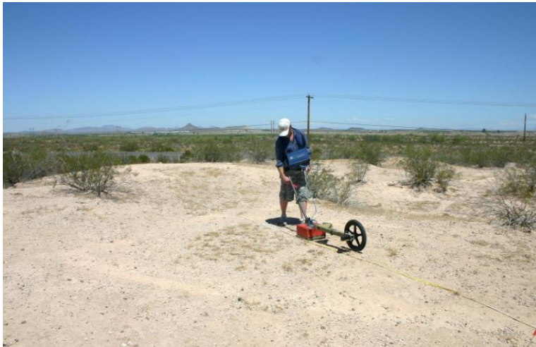
Collecting GPR data with a 400 MHz antenna, located in orange box, attached to a survey wheel for horizontal distance calibrations
