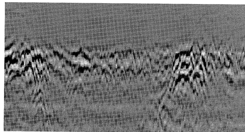
Figure 6. Reflection profile across a Great Kiva. The walls of the kiva are the high amplitude reflections, while the interior of the kiva is filled with wind blown sand, which reflects little energy.
