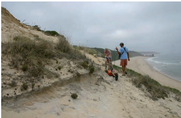
FIGURE 4 Collecting 400-MHz GPR reflection profiles in coastal sand dunes to produce images of the buried middle-Paleolithic soil horizon, visible just to the left of the GPR antennas in this photo.
