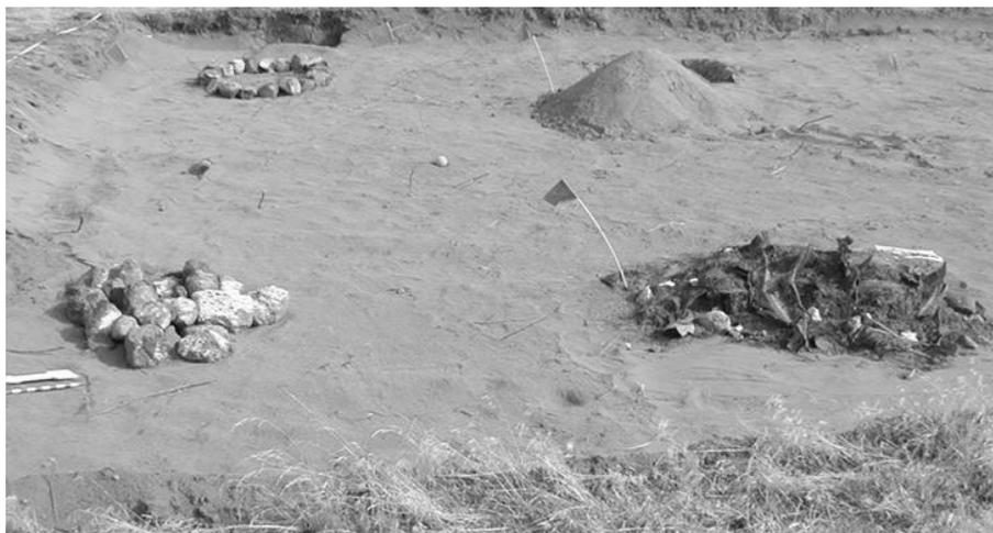
Fig. 8. Photograph showing the simulated shallow rock cairn, stone ring, brick well and trash midden, constructed at the 12-inch depth level of the Remote Target Test Bed. September 2002.
