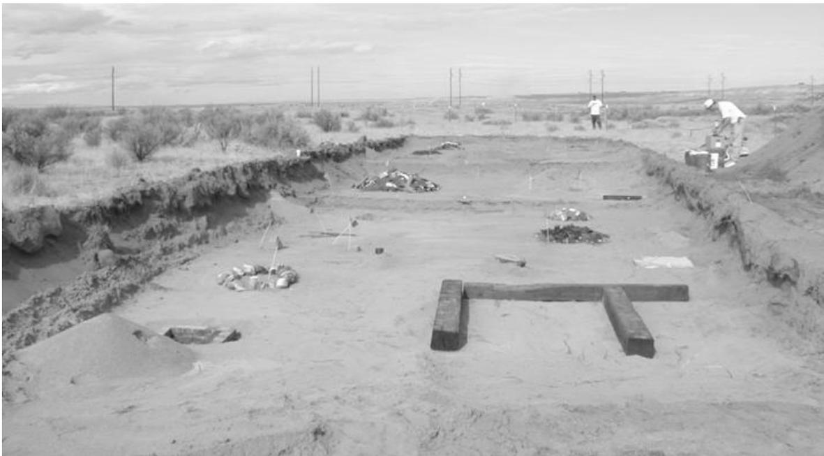
Fig. 1. The Remote Target Test Bed after trenching and placement of artifacts and features on the three excavation surface. The deeper zone (36 in.) is in the foreground, with the medium (24 in.) and shallow depth (12 in.) areas in the distance (looking north). September 2002.
