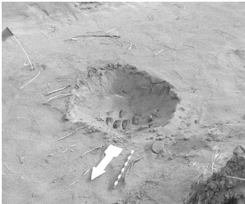
Fig. 10. Photograph showing the simulated cache of lithic materials, constructed at the 24 in. depth level of the Remote Target Test Bed. These small artifacts reflected no radar energy due to their small size.
