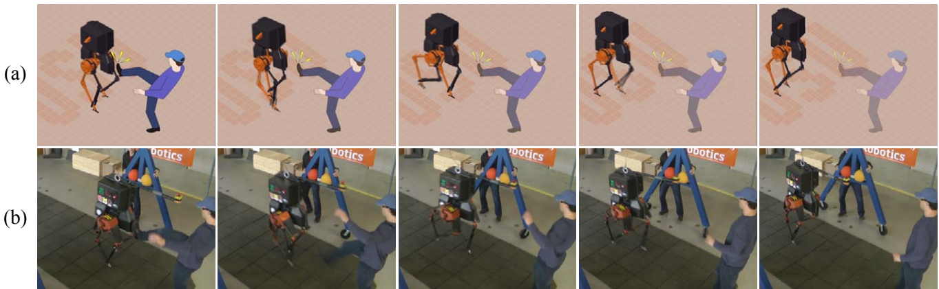
Fig. 9. Example of the use of full-body simulation in the development of ATRIAS' control. (a) A film strip of the SimMechanics model of ATRIAS, with hardware controller, being simulated with a large horizontal impulse (aesthetically illustrated with an overlaid kicking human). (b) Using the same controller, the physical robot is kicked to test its disturbance rejection.
