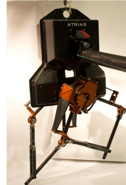
Figure 4. ATRIAS, a bipedal compliant robot
