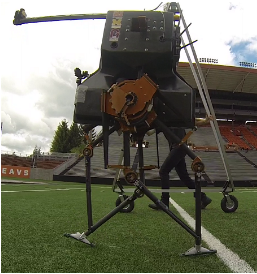
Figure 12. A snapshot of the robot walking/running at 2.2 m/s.
