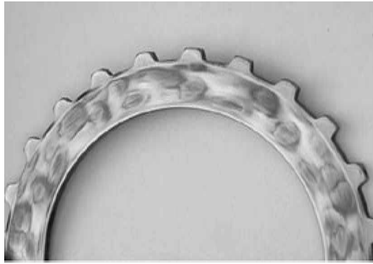
Figure 1. Evidence of hot spotting on a clutch disc.
