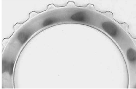
Figure 2. Clutch disc after a single engagement.
