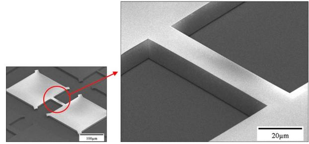
**Fig. 3** SEM image of the experimental setup of a MEMS beam resonator with a 0.5- $\mu\text{m}$  transduction gap.
