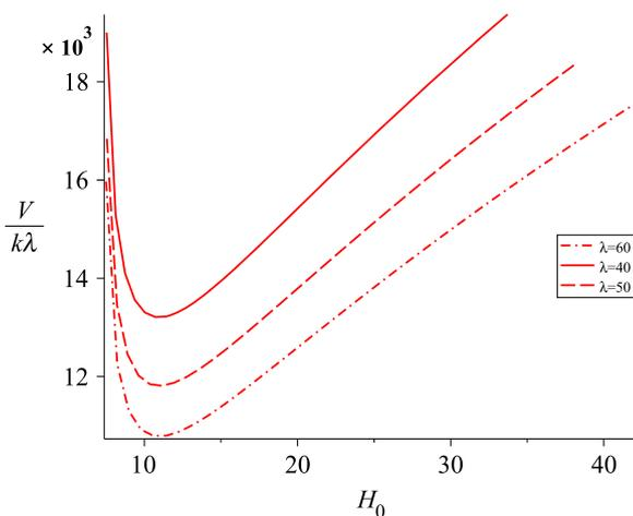
Fig. 7. The effect of the fluid film thickness on the critical speed.
