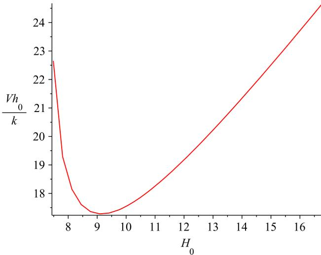
Fig. 4. The relation between the dimensionless critical speed and  $H_0$ .
