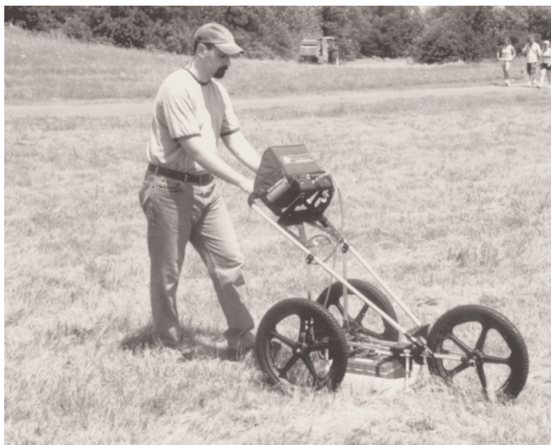
FIGURE 3.7 A One-Person GPR System. Some GPR systems can be mounted on a cart for one-person operation.
