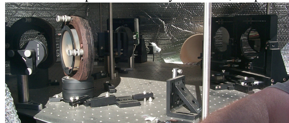
Figure 2. Optical bench within each of the huts, optics setup to correct for atmospheric aberrations, and a system of mirrors that convert the light collected to a collimated 4 inch beam which then
